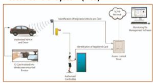
ACS is a vital contribution to building security and anti-intrusion in controlling entry or access to specific areas of the building. This may be from the main gate entrances for either vehicles or personnel via road barriers or turnstiles manually operated by security personnel or via means of a range of electronic technologies such as RFID cards that effectively act as an electronic key.
