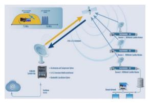
The VSAT is a system that uses a satellite as its communication link between two (2) or more geographically separated locations. We offer broadband internet services for areas that are beyond the reach of Internet Service Providers (ISP). An antenna system, usually a 1m dish antenna together with the IP satellite modem are installed in the client's remote location. From these, internet services are provided to the client's network.
