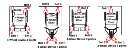
The illustration below shows how different types of mobility devices should be secured:
