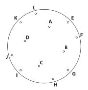
Long pendants hang around w/ central outlets ( A,B,C,D ) 內緣出線孔A,B,C,D吊掛較長燈球。
