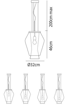
Glass diffusers can be arranged in four different positions, lighting source can be adjusted.
