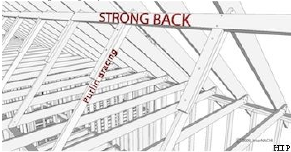
I observed the purlin was not flush with the rafter at the time of the inspection. A purlin is a horizontal structural member in a roof that supports a rafter. This was noted at multiple purlins in the back right corner when walking in through the front door.
