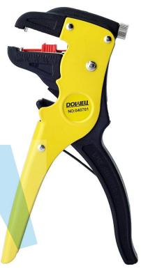
the knurled knob at the back of the tool head adjusts the wire diameter setting. Rotating this knob clockwise provides for stripping smaller-diameter wire, while turning it counter-clockwise sets the tool for larger-diameter wire.
