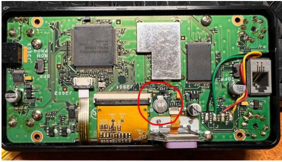
Figure 2 - Front panel coin cell location
