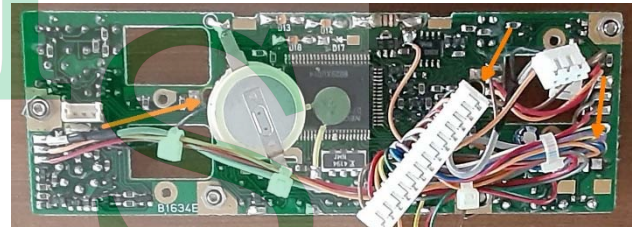
Figure 4 - Logic PCB with lamp holes indicated
