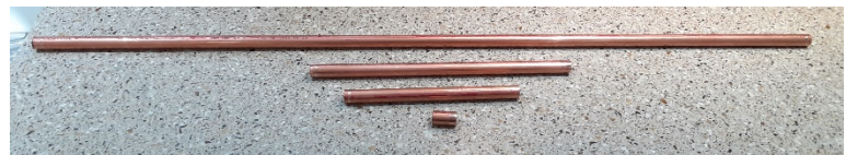
Figure 6 - Copper pipe cut to length
