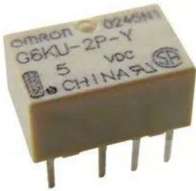
Figure 10 - Latching relay used
