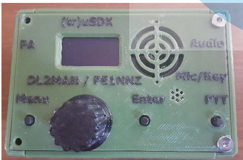
Figure 14 - All panels installed
