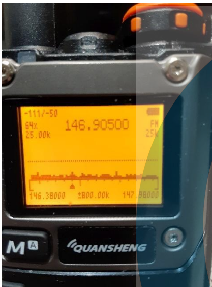
Figure 27 - Spectrum analyzer display
