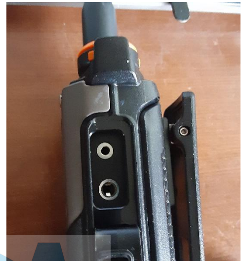
Figure 8 - Mic and speaker jacks on UV-K5(8)
