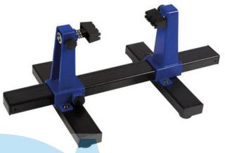
upright position to its inverted position and back again in a single direction is limited to those boards of five-and-a-half inches or less in width. This is not that great a limitation, though, as by installing a larger-width board in an offset position, it can be inverted though it cannot be completely rotated around its longitudinal axis.
