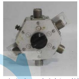
labeled "1" through "4", "C", and "G". The internal switching mechanism has no physical stop, which means that it can be rotated a full 360° if so desired.
