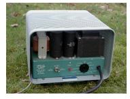
100mA, -100VDC at 20mA, and 12.6VAC at 5.5A. The incoming power is a standard 120VAC at about 350 watts. The unit is heavy, weighing in at about sixteen pounds.
