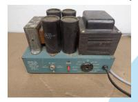
This particular HP-23B came to me with the complaint that it would repeatedly trip the chassis-mounted 2.92-ampere circuit breaker. The owner would press the reset button, and almost immediately it would trip out again. This behavior led me to believe that there was either a dead short circuit somewhere, or a condition that would mimic a short circuit very closely. Time for some detective work.
