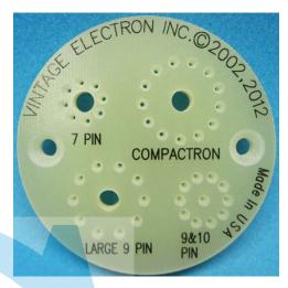
The tool is fabricated from a piece of one-quarter-inch thick FR4 fiberglass board material, and it is precisely machined as to its general form and its pin openings. Each of the pin openings is wider at the tool surface, where the pins get inserted, and then the holes taper down to the final pin diameter, bringing misaligned pins into shape quickly and easily.
