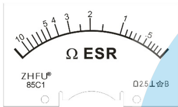
Figure 7 - Custom ESR meter face
