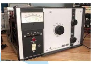
This was a circa 1977 model, heavier than you can believe, with a one-tube grounded-grid circuit. The tube is a 3Z500 tube of about four and a half inches diameter, nestled inside an external glass bell chimney. The tube socket is buried deep inside the unit, behind a board that carries the tuning coils for the amplifier.
