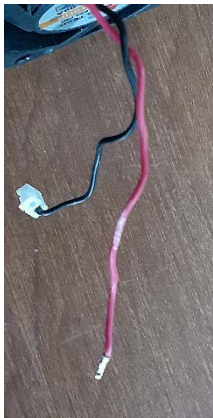
Figure 5 - Wire out for repair
