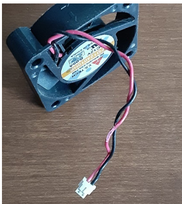
Figure 4 - Chafed area of fan wire
