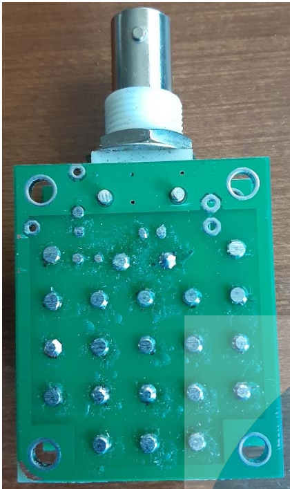
Figure 10 - Lower PCB after filing
