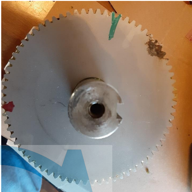
Figure 12 - Timing markings on output spur gear
