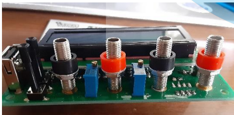
Figure 7 - Banana jacks ready for panel
