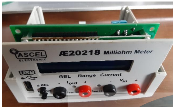
Figure 8 - Front panel and PCB installed
