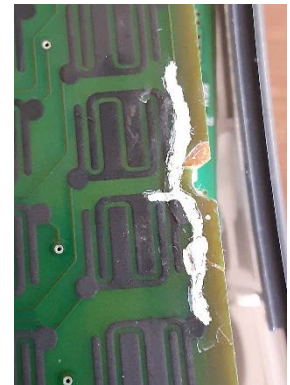
Figure 5 - Ink applied to PCB
