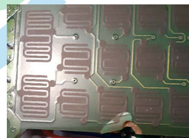
Figure 3 - Torn PCB traces
