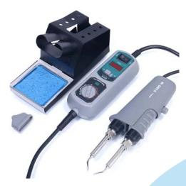
From time to time, it becomes necessary to solder – or desolder – SMD devices to or from a printed circuit board (PCB). While this can often be done with a pencil-type standard soldering iron with a fine tip, it is often much more convenient to use a pair of "hot tweezers" for this task.
