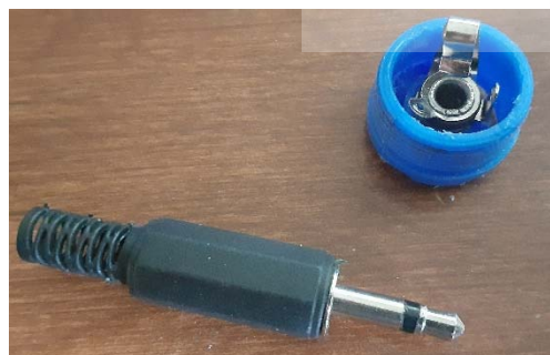
Figure 6 - Jack in end cap, with plug
