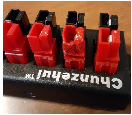
Figure 4 - Melted block port
