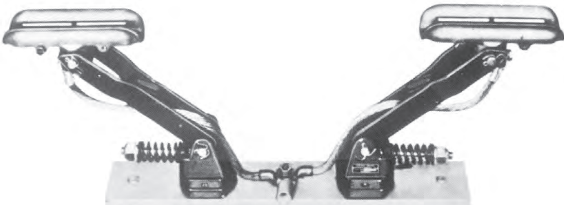
Typical arrangement of collectors in parallel
