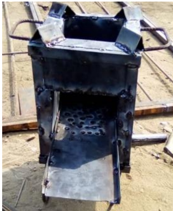
Figure 5. Fabricated Open Single Spout Stove
