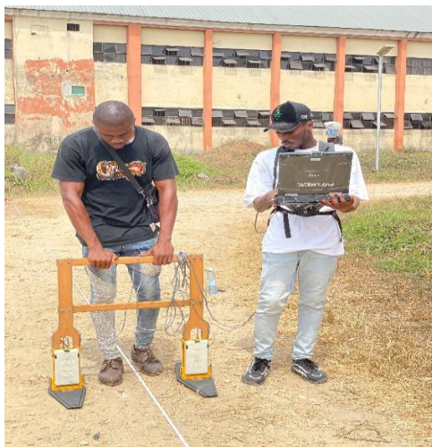
Fig 5: Field work on GPR Survey(Aurthors Fieldwork 2023)
