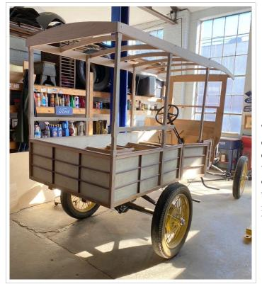
The construction of the Model T Depot Hack continues in Jim's Shop. Woodwork is nearing completion and almost ready for the clear varnish to be applied. Fenders have been ordered and the engine is built ready to install when the transmission is complete. Our goal is to drive it to the April Car Show at the White Home.
