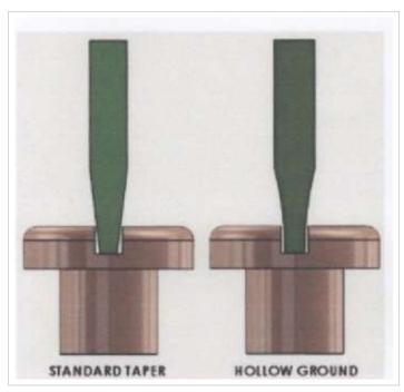
And don't forget about impact screwdrivers available for the really tough frozen screws. Most come with hollow ground tips and a tap with a hammer gives the force needed to break stubborn screws loose.
