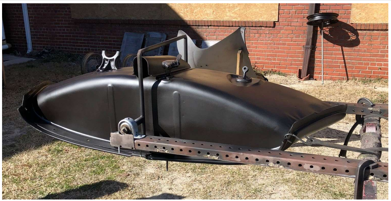
This shot shows the gas tank in the carriage designed to tumble the tank during cleaning. It served as a good holder during the blasting and priming process also.
