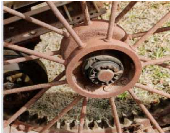
A pinion on the Model T rear axle engages the large internal gear on the wheel. The large gear reduction allows for a top speed of 5 mph in high gear!
