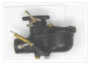
**Zenith Carburetors** - Cleaned, jets calibrated, and painted. New parts installed as needed. Perfect for touring or showing in touring class judging.
