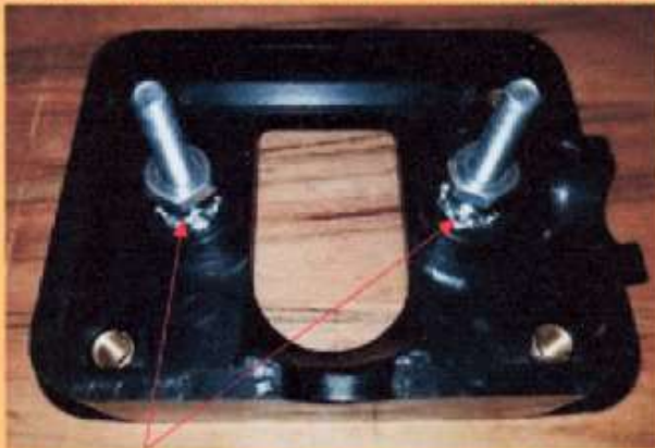
Two nuts are recessed into the box; the upper nuts secure wires
