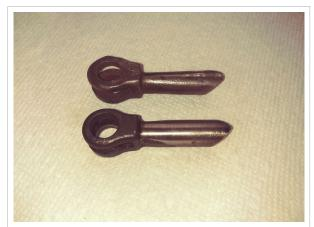
The adjusting shaft on the top of the illustration is the original. Note its diameter tapers from the tip to the base while the reproduction on the bottom is straight most of its length. The overall length of the two are the same but the camera prospective makes it look like the original is shorter.
