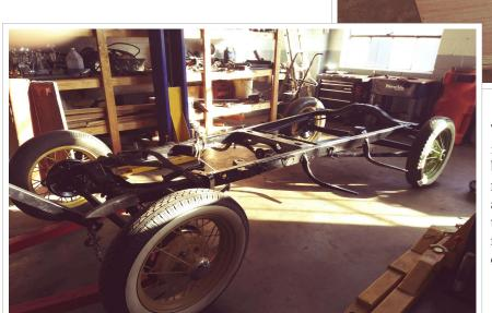
The chassis of the roadster project is nearing completion with the brakes reworked, the front end rebuilt, the rear spring reworked and with new shackles. The transmission has been rebuilt with new bearings and the engine is disassembled for rebuild.
