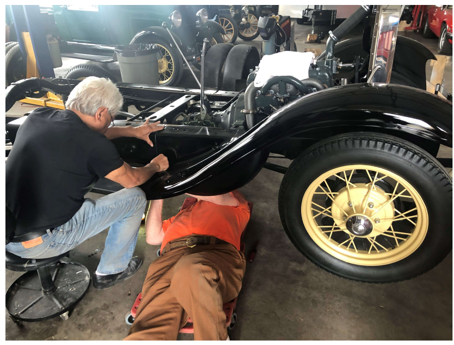
The front fenders and running boards are installed on the roadster project frame.
