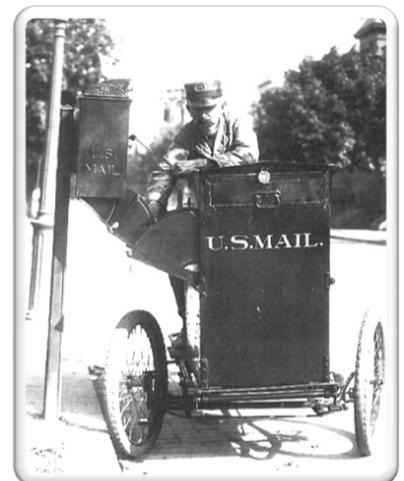
Photo from 1912 shows a motorized cart that was designed to receive mail from the boxes via a chute that dumped directly into the cart.
