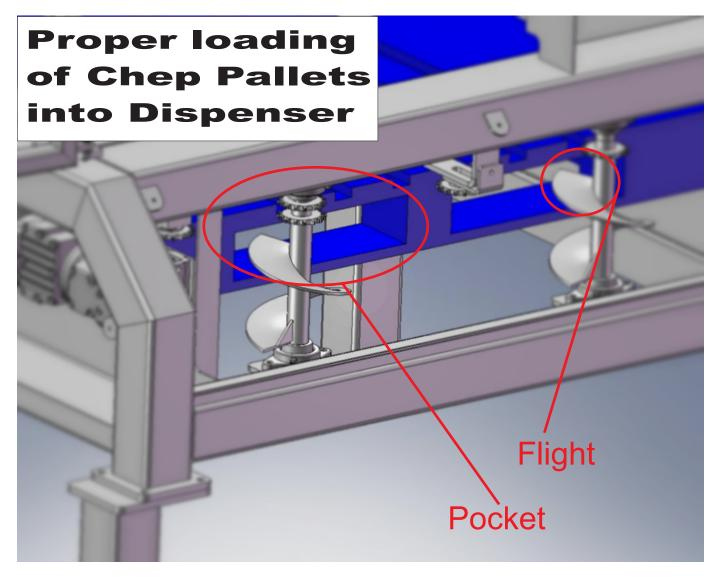
When loading Chep pallets into the pallet dispenser, Make sure that the top of the flight is engaged into the pocket of the pallet. If it is not, The dispenser will not feed correctly and cause unwanted jams.
