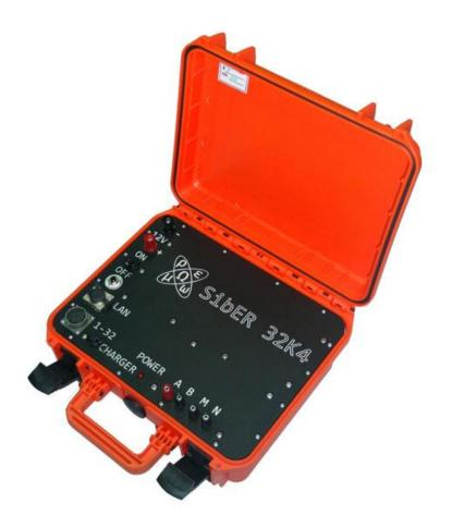
Multi-electrode geoelectrical solution SibER is meant to combine the functions of transmitter, multichannel receiver and switchbox in single protective case. The device is designed for electrical resistivity tomography (ERT) and vertical electrical sounding (VES) in IP or resistivity method. SibER can also be used for electrical logging. Our company manufactures reinforced sealed cable systems for electrical surveys with any electrode spacing that is perfectly compatible with SibER.
