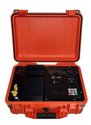
FastSnap is a multichannel automatically-controlled telemetry complex that ensures TEM/TDEM, frequency sounding, induced polarization and direct current techniques. The system is by far the most advanced in its class offering the highest technical specifications and most comprehensive software package along with an affordable cost. The software streamlines all aspects of advanced automated ground TEM survey.
