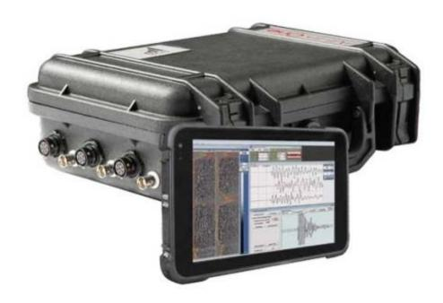
**All-in-One** is an easy-to-use non-destructive testing instrument with a multipurpose acquisition unit and specialized piezoelectric sensors that allows to perform sonic and ultrasonic tests for the characterization in situ and in the laboratory of materials such as concrete, masonry and stone materials, PIT and cross hole in piles and diaphragm foundations.
