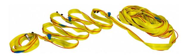
Towed LandStreamer is a receiver array, specifically designed for land seismic surveys. Towed techniques for land shallow seismic acquisitions significantly increase the efficiency and reduce the cost of the survey. Such methods as reflection, MASW, refraction would highly benefit from using towed streamer, comparing to the streamer with geophones, planted in the ground.
