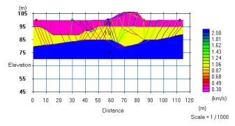
Set-up shots and receivers and perform a simulated survey. Adjust shot and receiver spacing to optimize coverage and minimize field time.
