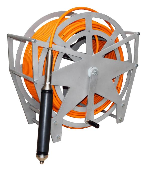
Borehole sparker **Pulse** is developed for generating high frequency pressure (P) waves in water-filled wells of up to 1000 m deep during crosshole seismic testing or tomography (<u>CST</u>), vertical seismic profiling (VSP) and other acquisition techniques with borehole source. The generation of polarized shear waves (SH and SV) is provided by sources <u>SHock</u> and <u>GeoSV</u>. All these sources require pulsed power supply <u>Jack</u>.
