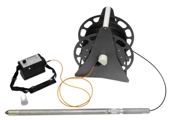
Borehole scintillation radiometer SRP-20 – the most advanced version of wellknown logging radiometers SRP-97K and SRP-68-02/03 and their analogue in terms of functionality and application. The device is designed to conduct gamma-ray logging in wells up to 300 m depth and drillings. The borehole and <u>hand-held</u> (analogue of SRP-68-01, SRP-88 and SRP-97) versions are in series production.
