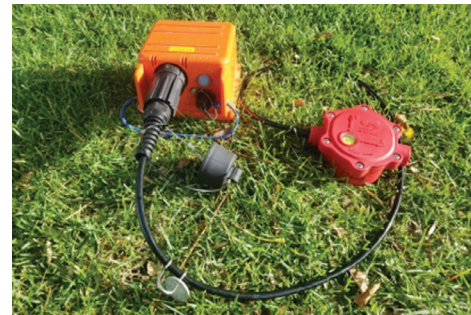
Atom-3C with 2 Hz triaxial geophone.
