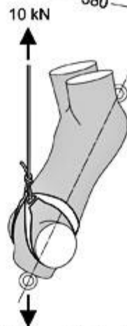
Strength test of chest harness
