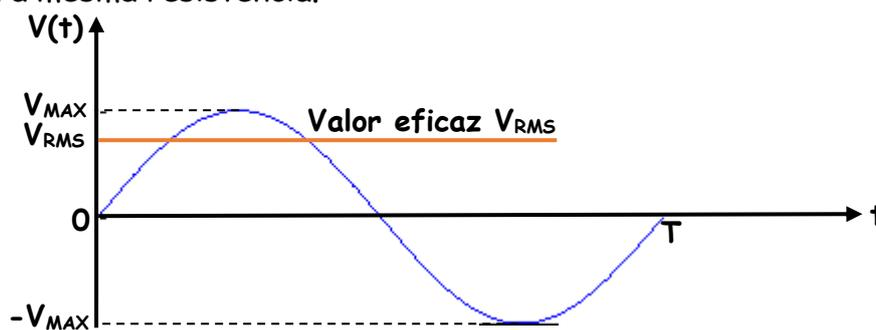
$$V_{RMS} = \sqrt{\frac{1}{T} \int_0^T f(t)^2 dt}$$
