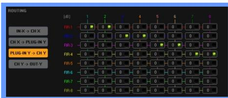
The output processing channel to the physical output channel can be superimposed on adjacent channels.
