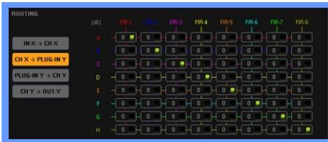
The plug-in channel to the output processing channel can also be sent in 8×8 matrix
