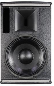
The NX12M is a compact yet high-performance two-way passive loudspeaker system. It features a 12-inch low-frequency (LF) driver with a 3-inch voice coil, and a 1-inch exit high-frequency (HF) compression driver equipped with a 1.75-inch titanium diaphragm voice coil. The NX12M's rotatable 90° x 50° HF horn ensures equal horizontal and vertical mouth dimensions, allowing precise directivity control in both planes.
